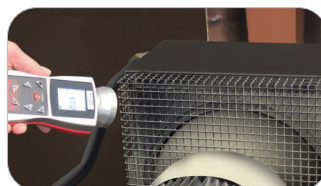
Stroboscope off: rotations not visible
