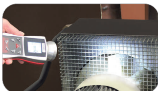
Stroboscope on: rotations visible
