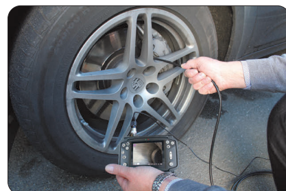
Example: brake discs control
