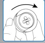
3. Lock the die by turning the retaining ring clockwise
