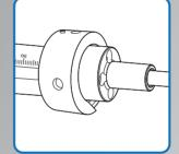
Start cutting the external thread by 3-4 threads
