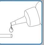
6. Lubricate bolt with sufficient cutting paste/cutting oil
