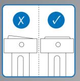
2. Make sure that the die is inserted in a straight position
