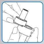
8. Turn back the SC adapter and remove the die guide
