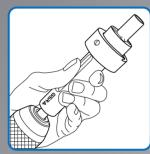
Clamp the SC adapter into the cordless screwdriver
