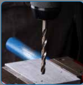
1. DRILLING FOR COUNTER SINK
