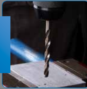
1. DRILLING FOR COUNTER SINK
